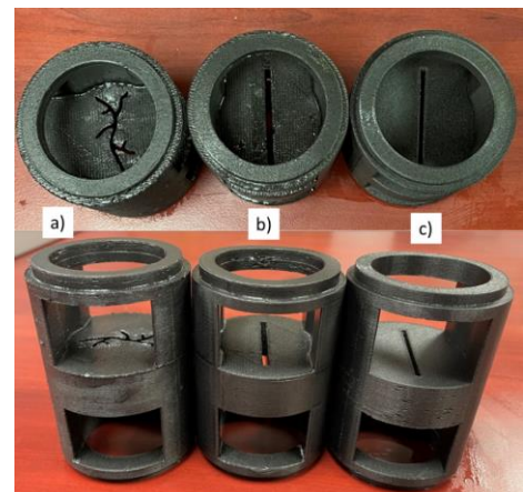
Figure 1 – 3D fractured discs used in this study: a) complex fracture, b) 3000 microns, and c) 2000 microns.
